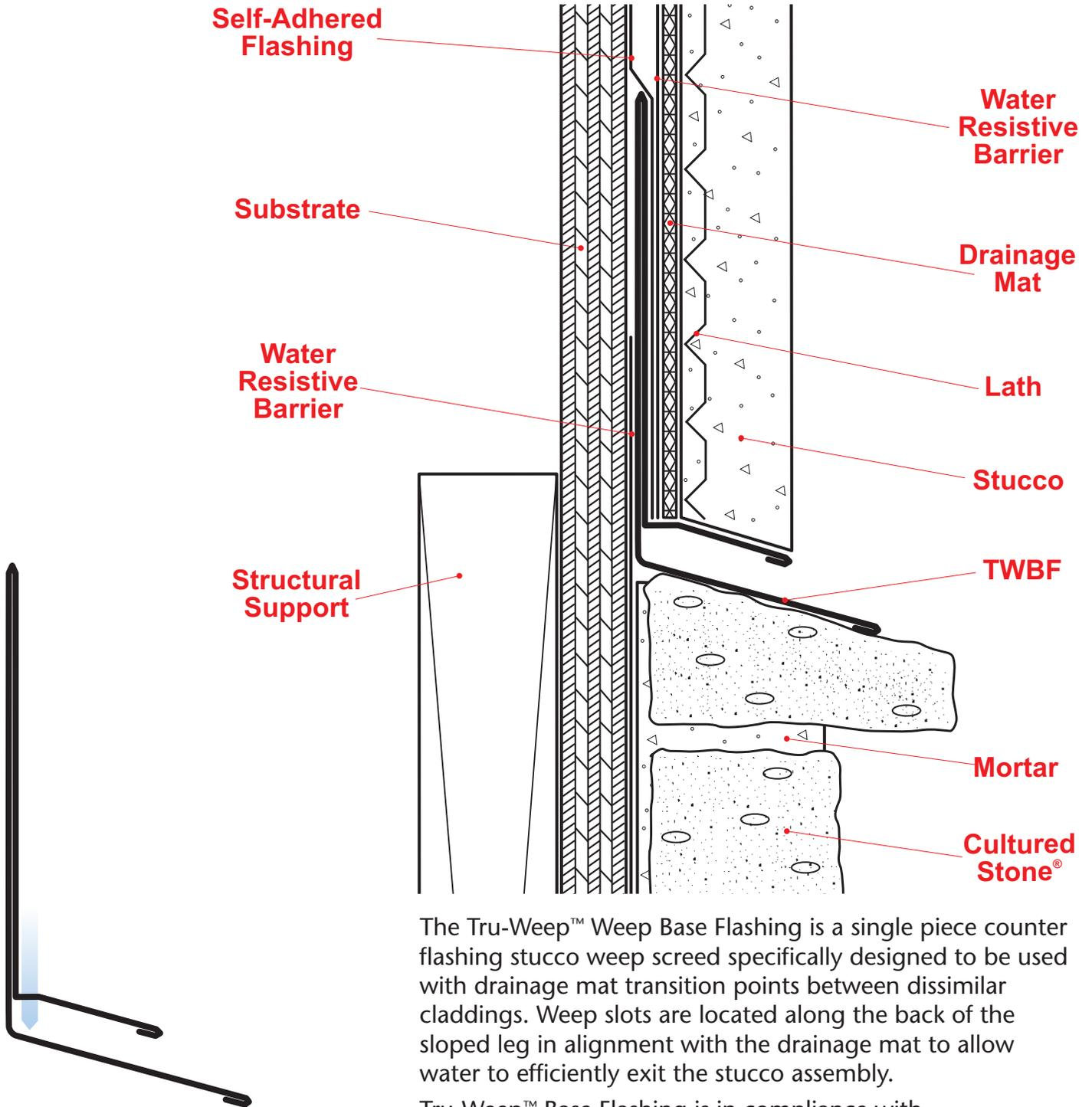
The Tru-Weep™ Weep Base Flashing is a single piece counter flashing stucco weep screed specifically designed to be used with drainage mat transition points between dissimilar claddings. Weep slots are located along the back of the sloped leg in alignment with the drainage mat to allow water to efficiently exit the stucco assembly.
