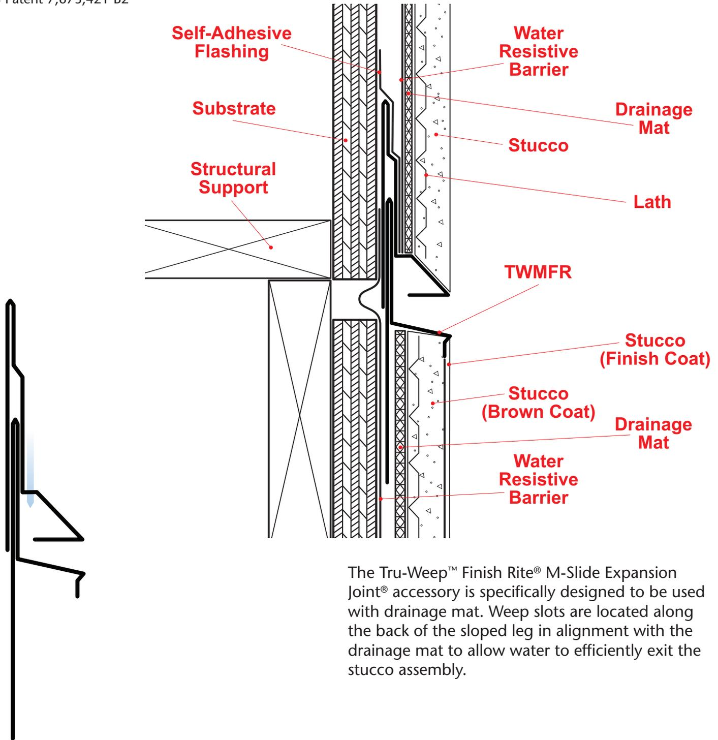
The Tru-Weep™ Finish Rite® M-Slide Expansion Joint® accessory is specifically designed to be used with drainage mat. Weep slots are located along the back of the sloped leg in alignment with the drainage mat to allow water to efficiently exit the stucco assembly.
